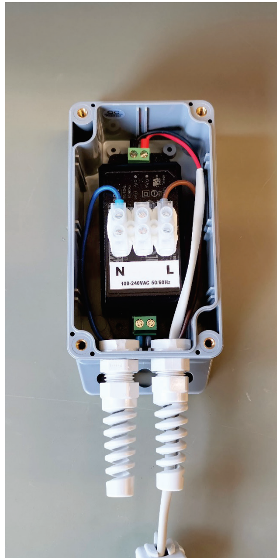
Figure 4: Connection terminals for connection to the mains voltage in the supplied power supply
